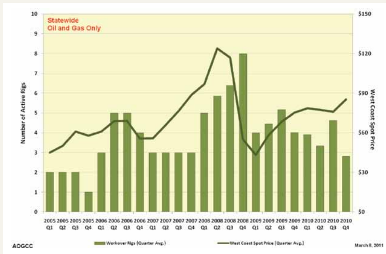
Figure 4-3 Alaska's active workover rigs for each quarter from 2005 through 2010. Solid line represents West Coast spot price for Alaska North Slope crude oil (dollars per barrel)
