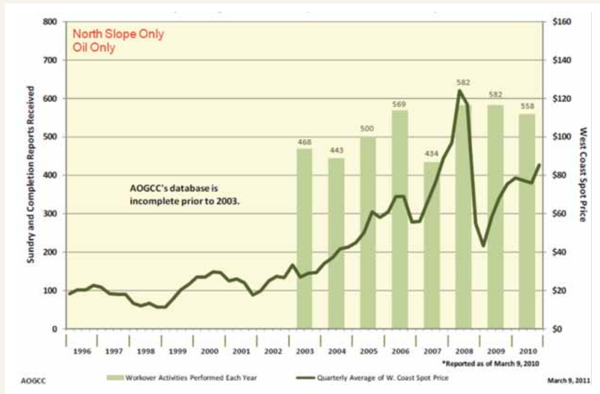
Figure 4-4 Number of Alaska's well workover activities by calendar year, North Slope only, from 2003 through 2010.* Solid line represents West Coast spot price for Alaska North Slope crude oil (dollars per barrel)
